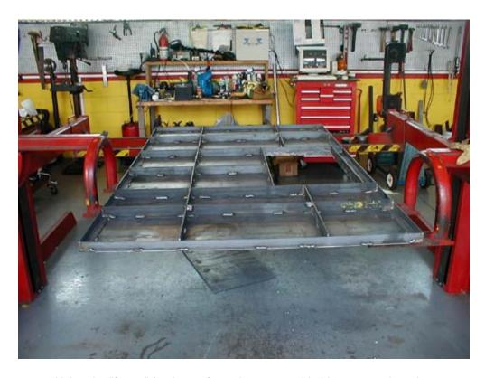
Using the "frame" for the surface plate as a guide I just cut on the edge and then ground the cut smooth.
