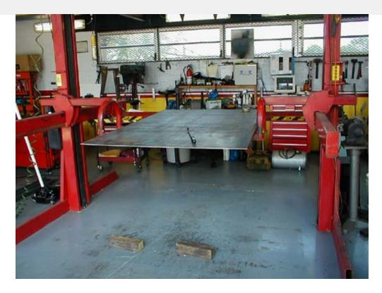
This is how we began. It's 1/4" sheet cut to the same dimensions as the original table. Here it's setup on the lift arms of our lift, not the ideal setup but better than bending over on the floor.
