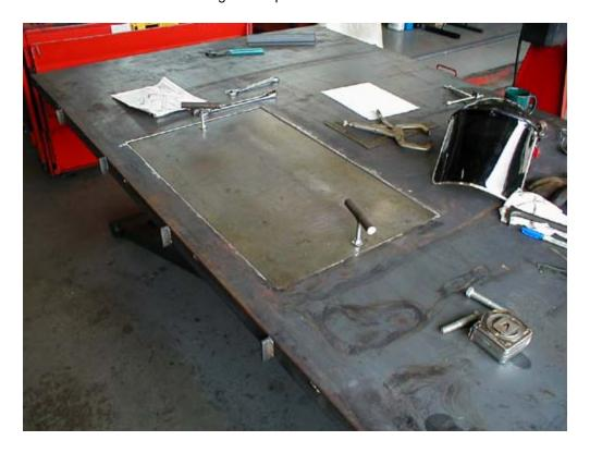
This is the top with the surface plate installed and I'm working on the guardrail. The surface plat is about 16 X 24 and 1" thick. It's machined to .002 on both sides (one's a spare). I drilled and tapped it so I could put some handles in it. My thinking there was we could take it to the machine for a quick setup if needed. It also makes it easy to move.
