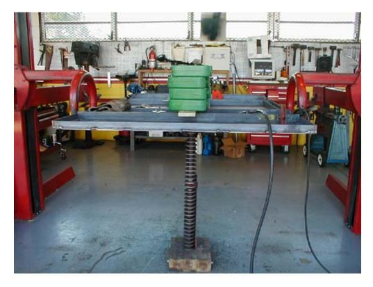
This is how we "make do" when there's warpage. The table is lowered on a roller and tractor weighs are put on top. Then it's tacked.
