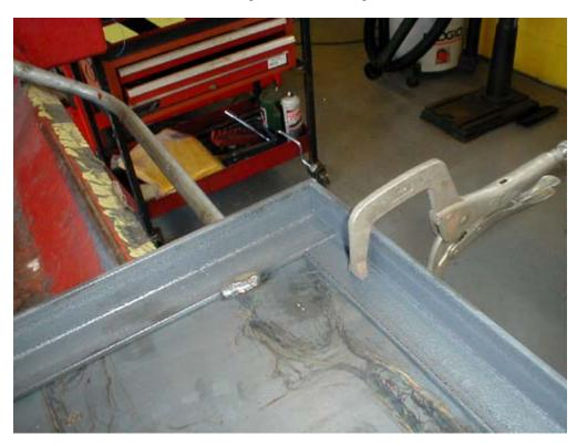
Usually I'm trying to get things done fast so corners have not been as nice as I'd like. Here we've just notched the angle on the bandsaw. Very quick and a nice fit.
