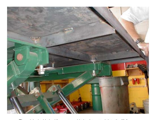
The original table had four nuts welded to it to attach it to the lift frame.
