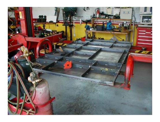
The cross bracing is 2 X 1/4" flat stock, the layout is fairly close to the original table. I really want to be able to abuse this table and don't want to have any problems later on due to a "strength" issue so I probably went overboard a bit on this.
