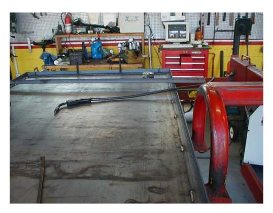
Here I've started welding 1-1/2 X 3/16 angle iron as a frame.
